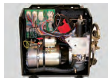
LOW NOISE POWER UNIT & NO ELECTRONICS = EASY MAINTENANCE
