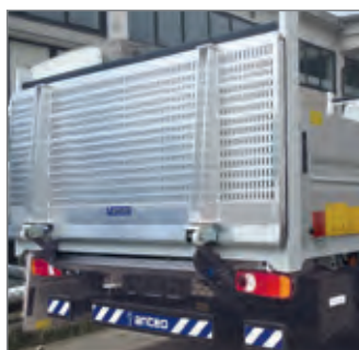
38 Perforated premium aluminium platform.
