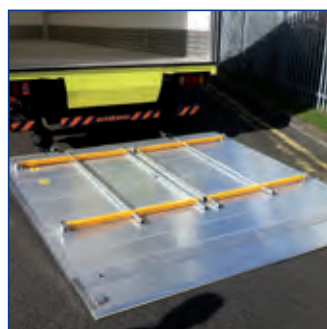
Guard hinged and folding on platform.
