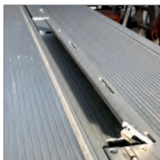
28 Automatic trolley stop 45° (2 stops).
