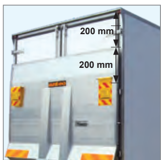
34 Aluminium platform extension (for each 200 mm).
