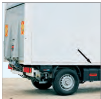
21 Removable hydraulic power pack not integrate with the lift.
