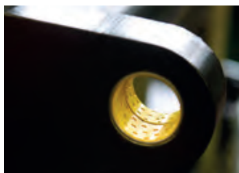
LOW MAINTENANCE BUSHES AND CHROMIUM PLATED PINS.
